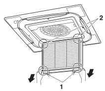
1 Pull the air filter end inclined downward and unhook the hooking hole of the air filter from the projection of the grille. (both right and left)
