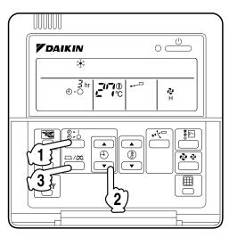
1. Press the TIMER MODE START/STOP button several times and select the mode on the display.
