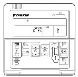
Press the AIR FLOW DIRECTION ADJUST button to select the air direction as shown below.
