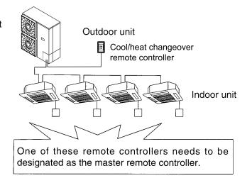
• The displays of slave remote controllers show " \[ \] \( \) \( \) (CHANGEOVER UNDER CONTROL) and they automatically follow the operation mode directed by the master remote controller. (This symbol is not displayed in wireless remote controllers.)
