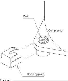
If the unit is operated with the shipping plate still attached, abnormal vibration or noise may be generated.
