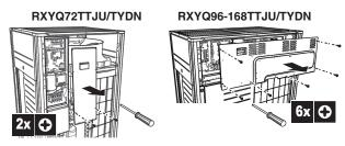
For service purposes, the push buttons on the main printed circuit board need to be accessed. To access these push buttons, the control box cover does not need to be opened. See 13. Making field settings on page 23.
