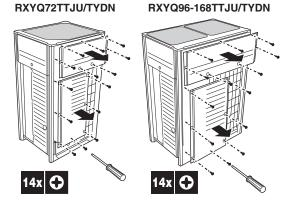
Once the front panel open, the electrical component box can be accessed by removing the control box cover as follows.
